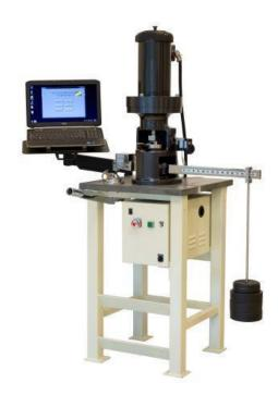
The Falex Four Ball Extreme Pressure Test Machine measures a lubricant's extreme pressure properties under High Hertzian contact in pure sliding, or pure rolling motion. The test is used to determine the load carrying properties of a lubricant at high test loads. The Falex Four Ball EP Test Machine is available in two configurations : Standard System and High Performance System with Data Acquisition.
